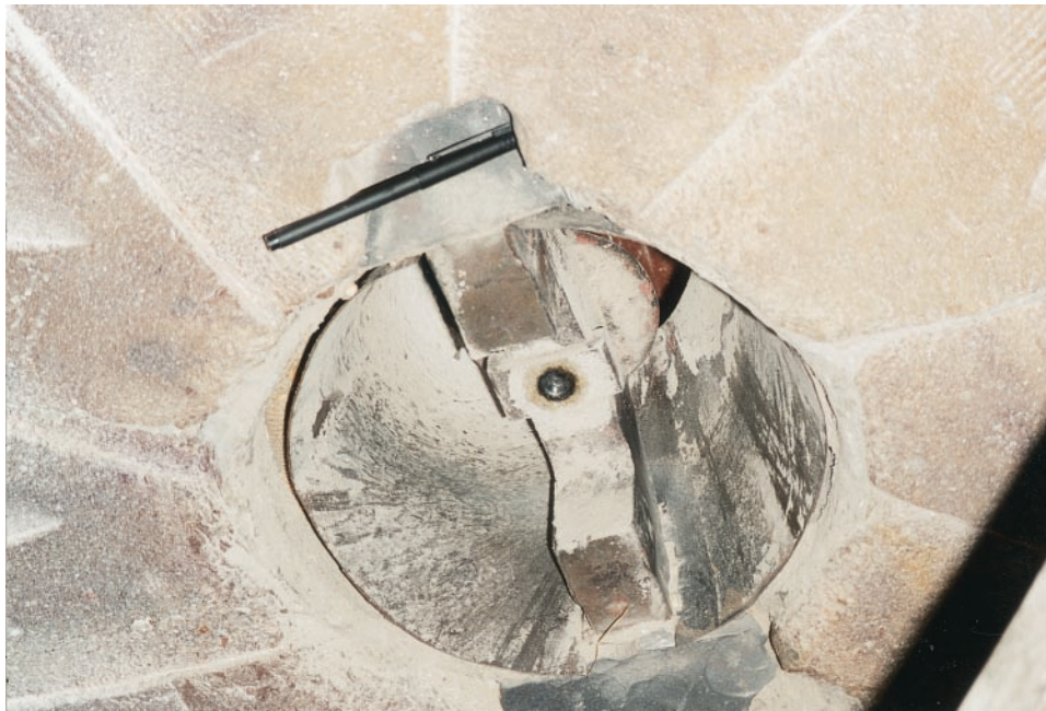
Fig 2. Upper grinding stone turned over, showing molten lead (see pen pointer) used to attach stone to iron bar that is turned by axle/diesel motor.
